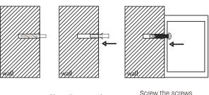
Drill Hole Place the expansion tube into the hole
